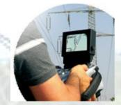
The Ofil DayCor® Superb<sup>™</sup> Corona Camera is the perfect tool to use to detect Corona and Arcing on Overhead Transmission lines and in Substations. Detect Partial Discharge and arcing on large Generator or Motor Stators and other HV equipment. Use for detection of dry arcing on ceramic and glass insulators.
