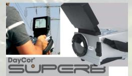
The DayCor® Superb<sup>™</sup> technological innovations include such exclusive items as dedicated **Quartz Catadioptric optics** with fast auto-focus, proprietary Lindner UV filters and high quality surface mount components in a light weight carbon fiber body. **Human engineering design allow for Teamwork with perfect group viewing of corona events as an important feature!**
