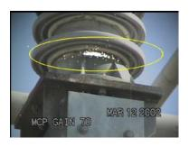
The two pictures to the right show severe Corona on a **NCI Polymer Insulator**. The left picture vividly shows the Corona discharge with medium gain of 180. In the right picture the gain has been reduced to **pinpoint the exact location of the problem!** Observe the high Corona photon count. This insulator needs to be replaced and the replacement unit needs a corona ring! The camera gain setting goes from 0 to 250.
