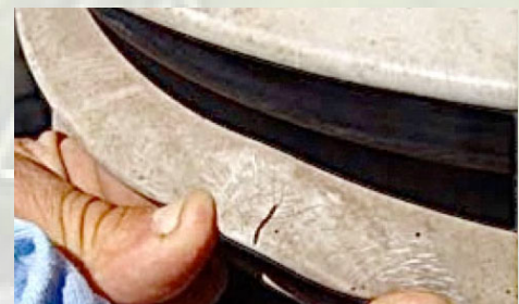
Above: Brittle non-ceramic bushing causing Corona
