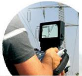
The best way to find Electrical Corona Discharges on High Voltage Overhead Lines, Transformer Bushings, Breakers and more is to use a very sensitive Corona Camera.
