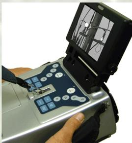
**Digital Video and Voice Recording plus Snap-Shot image Recording** is provided in the camera and stored on a removable SD flash card. **Playback and review function** of video and pictures is included in camera!
