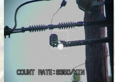
As fall weather is upon us with higher humidity and changing temperatures, chances for Electrical Corona on High Voltage overhead lines and substations increases! Contaminated or faulty insulators and missing or damaged hardware could produce a dangerous Corona event with resulting flash-over conditions.
