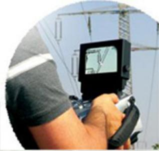
The best way to find Electrical Corona Discharges on High Voltage Overhead Lines, Transformer Bushings, Breakers and more is to use a very sensitive Corona Camera.
